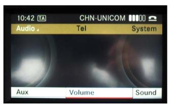
**6)**Now the original COMAND controller can control the Main Interface. If want to go to the original car system, you can long press on the "C" button which on the right of the original COMAND controller about 3 seconds .
